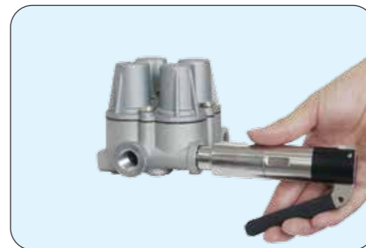
2. 松开压柄 (按钮、手柄), 螺纹卡爪膨胀, 锁紧螺纹, O型圈密封端口 Release lever(button, handle), thread collets expand, lock thread, O-ring seals the port
